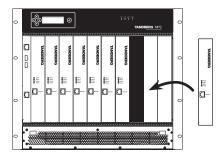
Insert the new Gateway board into the first available slot in the front panel.
